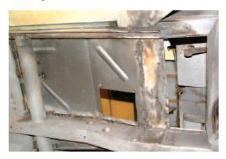
Objective – to remove all components, filth, materials, coverings and paint which are required prior to separation of the outer body shell from the chassis assembly. First stage of the strip is to remove all interior trim and glass, labelling and carefully storing. Next follows bumpers, all bright trim, light fittings etc. Next the transmission tunnel was removed followed by the removal of radiators, engine and transmission in unit, initially to be stored and later assessed.
